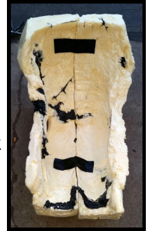
Seat in two-halves ready for covering. Photo by Larry Mason
